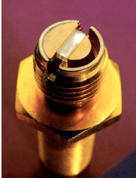
Figure 6: Photograph showing a diamond radiation detector. The diamond element is mounted within an SMA connector.
